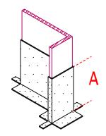
Step 2. Cut, Fold & Apply finger flashings at column web for both sides
