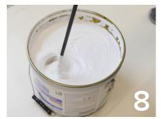
8. Thoroughly stir the entire container of Forti-Lock resin using a slow-speed mechanical mixer for two minutes prior to each use. Mix with spiral agitator or stirring stick, taking care not to aerate the material.
