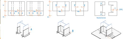
7. Dry fit Forti-Lock Reinforcing Fleece around penetration prior to mixing and applying with Forti-Lock resin.
