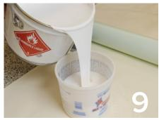
9. Pour resin into a secondary container used for measuring and/or mixing. Catalyze only the amount of material that can be used within 10-15 minutes.
