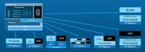
ZF DIV-A Software Platform Concept with Stepwise development and Stepwise integration allowing testing in early phase and independent development
