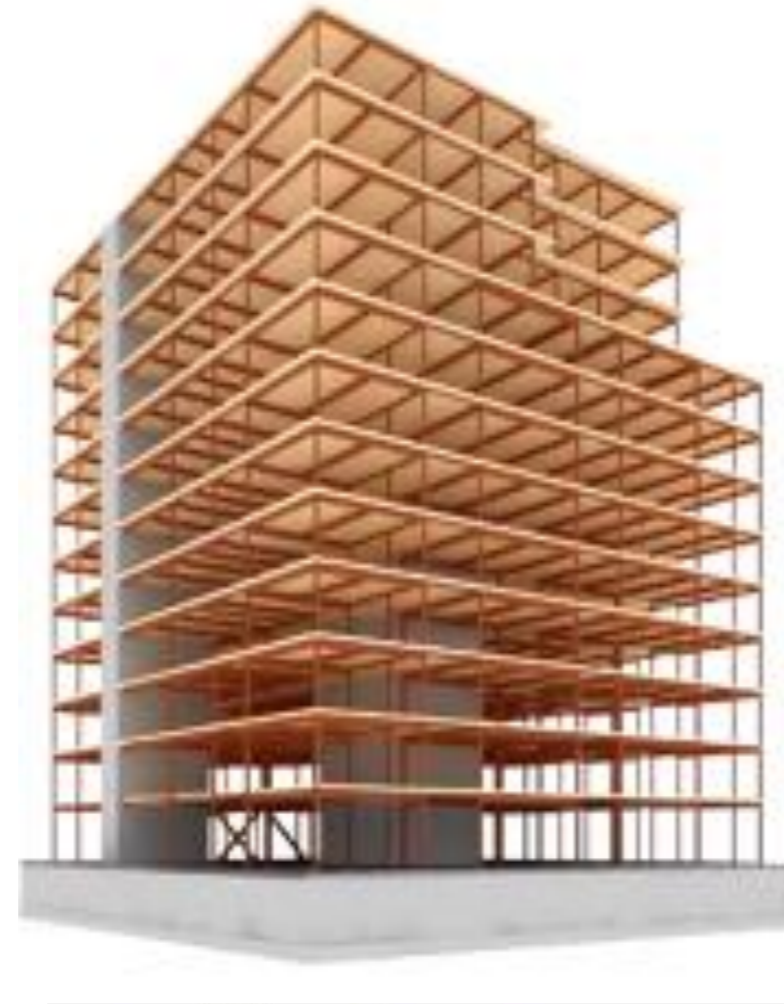
Steel Frame + MT Floors Hybrid 9 - 15 bf/sq.ft.
