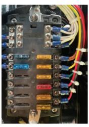
PANDO **FUSE AMP DESCRIPTION** 15 Stereo 5 **Exterior Lights** 15 Fridge 3 Interior & Galley Lights Optional Fridge 5 15 5 USB Plug **Empty** 10 Water Pump 9 **Empty** 10 5 Fan 11 **Empty** 12 **Furnace**
