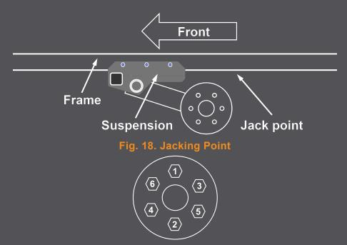
Fig. 19. Wheel Lug Nut Tightening Pattern
