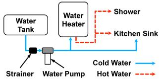
Fig. 21a. Water Heater General Layout
