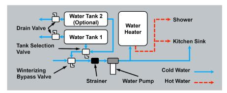
Fig. 21c. Water System Layout - Pando
