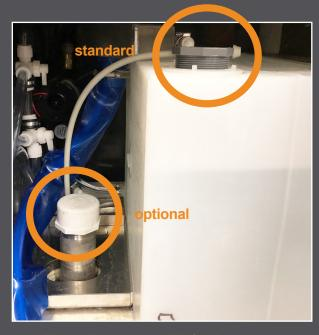
Fig. 6. Freshwater Fill for Pando 2.0
