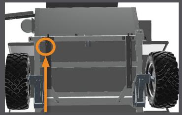
Fig. 7. Freshwater Drain for Expedition 2.0 is under the rear drivers bumper
