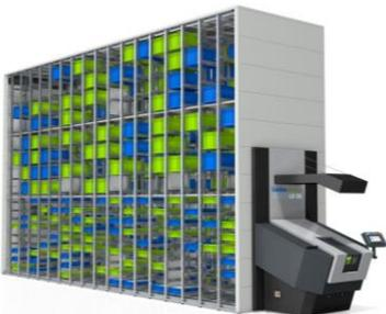
**Vertical Buffer Modules (VBMs)** – In the middle of a multi-segment shelving system is an aisle, where a moveable mast with a telescopic gripper operates. The control unit sets the gripper in motion picking a bin and transporting it to a picking station.
