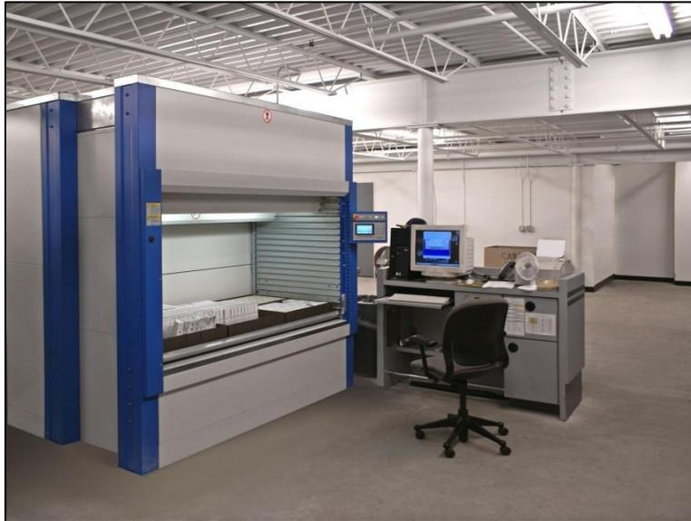
If a requested part is located in bin storage, a clerk on the second-floor mezzanine delivers it to the first-floor parts department using an open tray in the Shuttle XP VLM, eliminating the need for additional personnel to move parts between floors manually.
