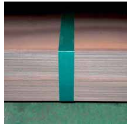
Strapping of steel plates
