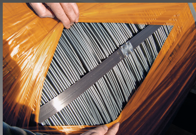
Metal after transport with MetPro VCI protection
