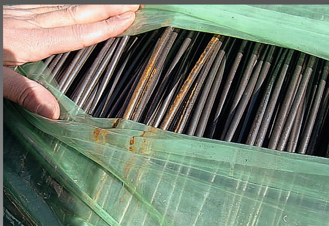
Metal after transport without VCI protection
