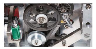
Free Access to Strap Guides <sup>(patents registered)</sup> Hinged top plate makes easy access to the strapping head for quick maintenance. Unblocking the guides enables free and quick access to strap guides without using any tools. The most maintenance friendly design.
