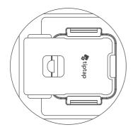
Pull out rubber cap from the battery pack and plug it into the device.
