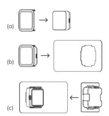
Peel off double sided tape covers on the back plate and attach it at the back gasket.
