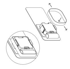
Peel off double sided tape covers on the back plate and attach it at the back gasket.
