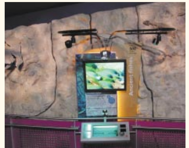
The ramps that lead visitors down the Deep include many interactive exhibits like this one that includes a touch screen, a plasma display, and an overhead parabolic loudspeaker to confine sound to the immediate exhibit area. The company Atacama was responsible for video programs and computer-interactive software.
