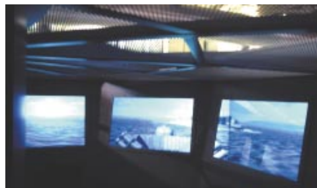
This Ship's Bridge simulation at Action Stations runs a five-screen sequence from an Electrosonic multi-channel video server. The original material was generated on a real simulator, but is here run as an automatic show. ESCAN™ keeps the show in sync, and ensures that the projectors have the correct power-up and power down routines to achieve maximum lamp life.
