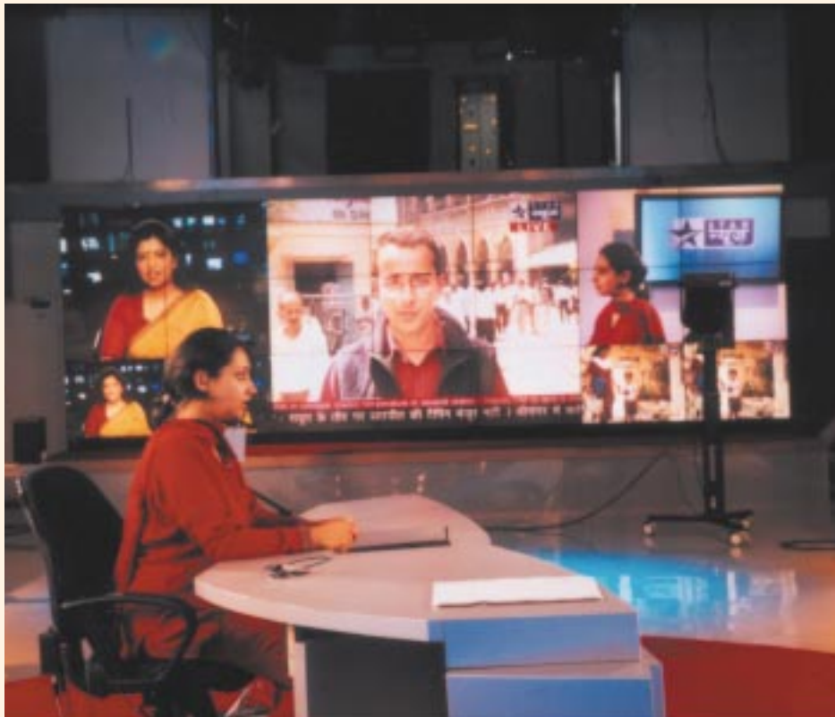
The videowall used in Star TV's Mumbai studios is made up of an array of 7x3 screens to achieve a display 24ft x 7.75ft (7.3m x 2.35m). It uses a frame construction developed by Electrosonic Systems Inc for permanent installations. Each screen module is 53 inch diagonal, and the projectors used are Pioneer videowall "engines". Photo by Alec Wood.
