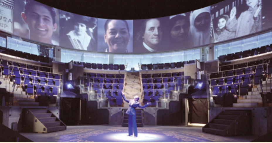
The “Freedom Rising” show uses 10 projectors sourced by a multi-channel video server to produce a 360° image. In addition Electrosonic HD players are used for the “floor” image and for four gauze screens that appear during the show.
