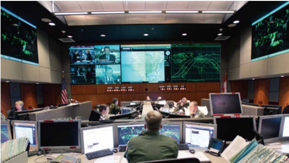
At the NORAD Command Center 12 Clarity LION 67 inch and 16 PUMA 50 inch UXGA displays are used with Electrosonic VECTOR™ image processing.
