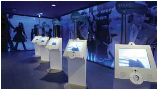
The log-in stations. Notice the camera above and the RF tag reader below the screen.
