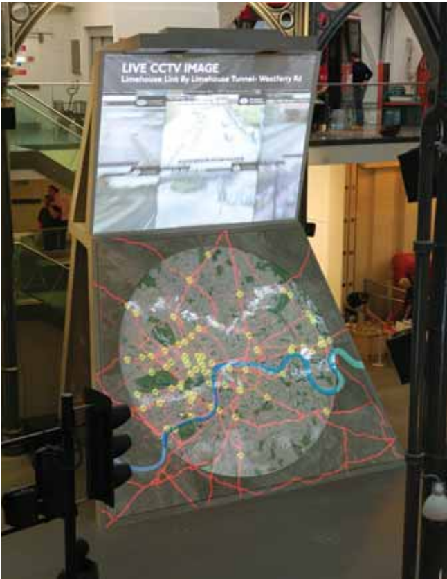
“Connections” features a 4m diameter 3D model of London, surmounted by a large projection screen showing live video images. Actual commuter routes, matching the overhead images, are projected on to the model. Photo: Andy Paradise. Copyright: London Transport Museum.
