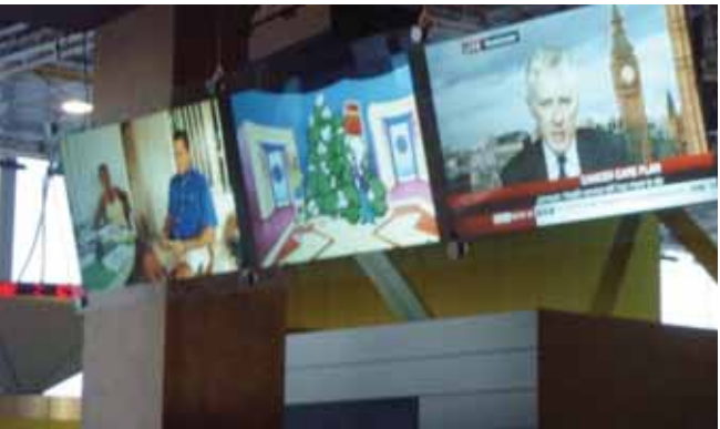
The “monitors over” exhibit shows high contrast images in high ambient light. Glass rear projection screens with 3M Vikuiti™ black film are used.
