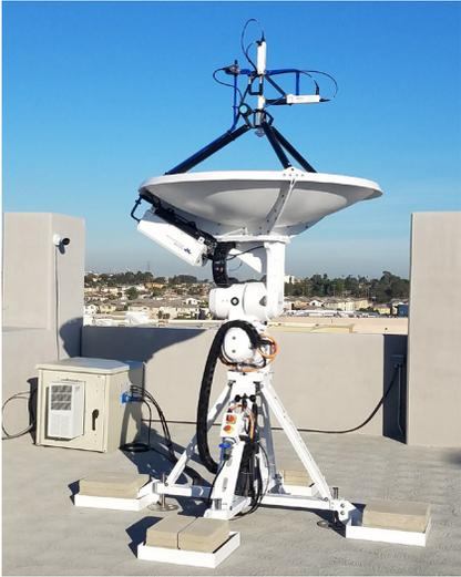
Modular Type 1 Deployable with non-ground penetrating mount
