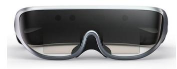
Voler worked with Rokid to create the entire electronics design. We integrated multiple sensor technologies—HD Camera, Time-of-flight camera (3D), audio (play and record), and included WiFi and Bluetooth connectivity. There is an HD video display projected on the lens in front of your eye. Given the multiple use cases planned—from mission critical tasks to hands-free operations, the battery life was critical and we were able to deliver a custom board that just sipped power.
