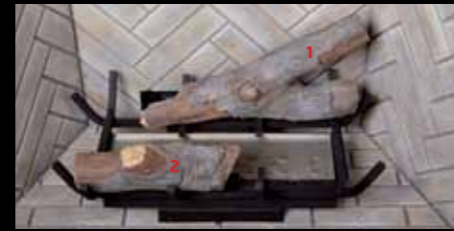
C. Place #2 log on the front side of burner towards the left with knot facing up and slightly forward.
