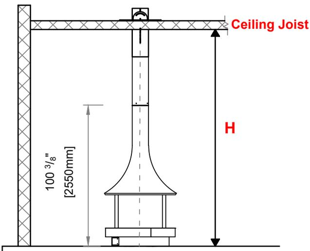
NOTE: Only the hood and extension pieces hang from the ceiling. The fireplace and base mount to the floor. The fireplace must not bear any weight.
