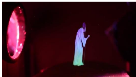
Projection onto particles optically trapped and moved by a UV laser, BYU, 2016
