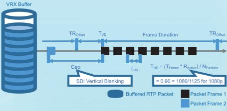
The Gapped PRS for progressive video contains a time gap between frames when no packets are sent. This allows delivery of video frames with an approximation of an SDI blanking period. The calculation of the packet spacing T<sub>RS</sub> changes slightly from the Linear PRS due to the gap.
