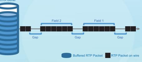
The **Gapped PRS for interlaced video** contains a time gap between each field when no packets are sent, which approximates to an SDI signal with a blanking period.
