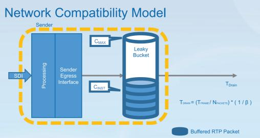
The Network Compatibility Model ensures that the IP network can cope with a large number of simultaneously converging SMPTE ST 2110 streams without switch buffers or queues overflowing. It is based on the leaky bucket algorithm, with packets being drained on a regular basis.
