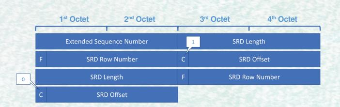
The ST 2110-20 RTP payload header begins with the 16 high order bits of the extended 32-bit sequence number, providing support for RTP packet re-ordering over a longer period. It also contains one to three SRD headers, which contain SRD Length, SRD Row Number and the field identification flag (F). Each SRD header refers to an SRD segment that follows the RTP payload header.
