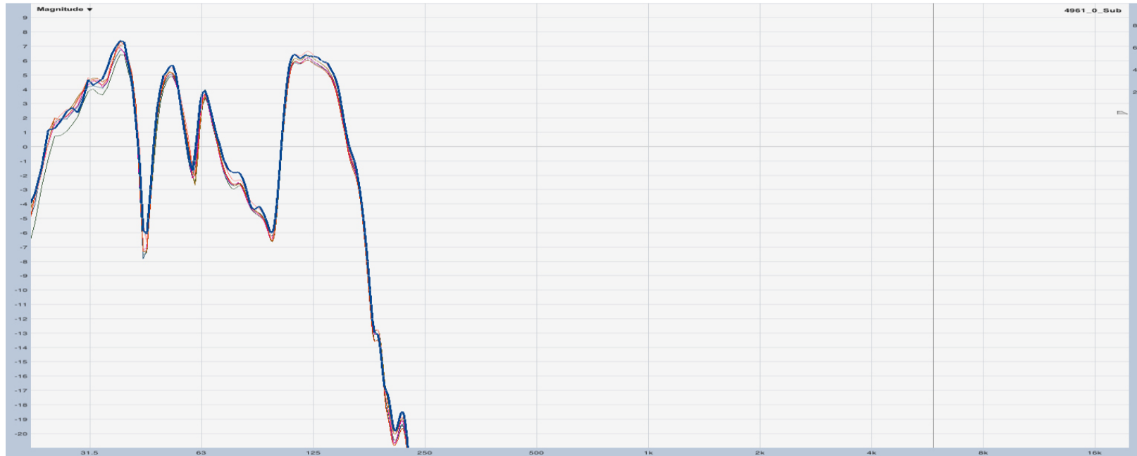
Figure D. 3 – Microphone Comparison - Sub-woofer - 0 degrees - 1/24 octave smoothing (Reference Screening Room)
