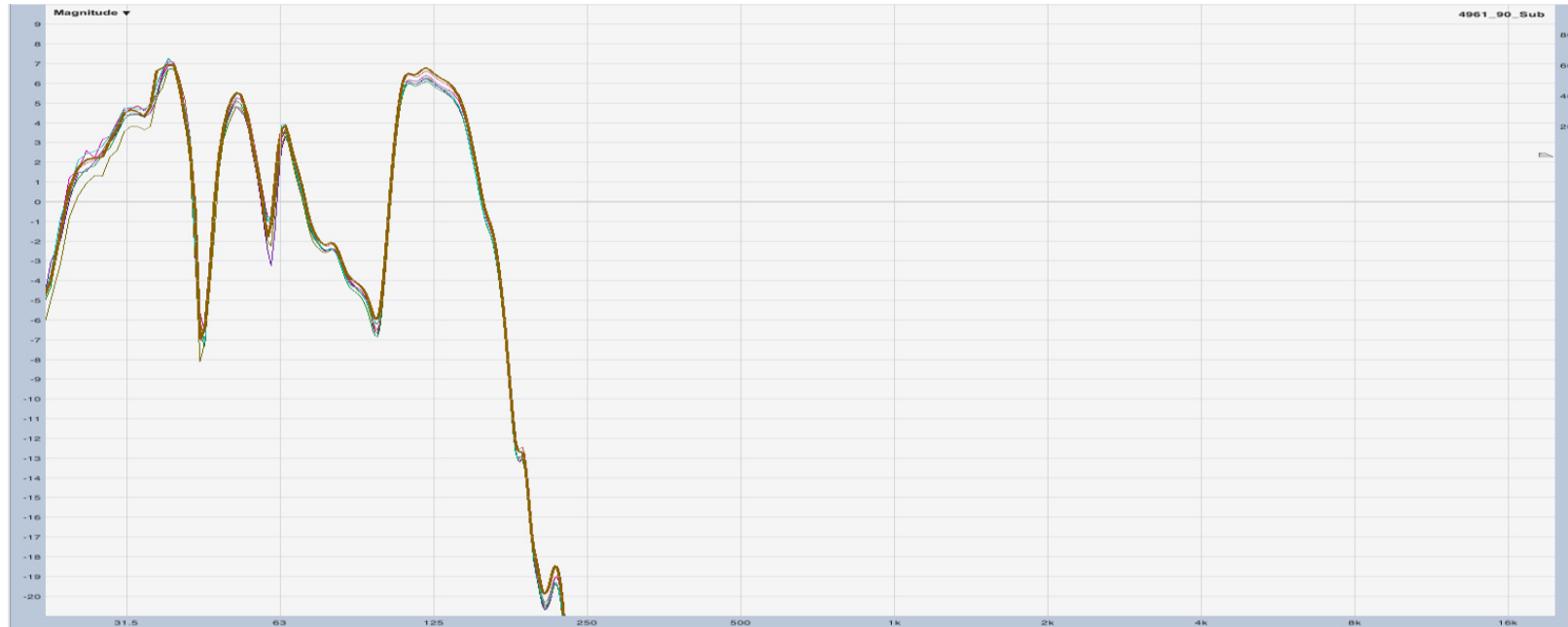
Figure D. 4 – Microphone Comparison - Sub-woofer - 90 degrees - 1/24 octave smoothing (Reference Screening Room)
