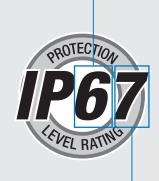
The second number listed after the letters IP= the level of protection against liquids. In this case, the number '7' indicates protection from temporary immersion in water of up to 1 meter for up to 30 minutes at a time.
