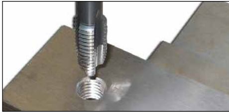
A TAP IS USED TO CREATE THREADS IN AN EXISTING HOLE
