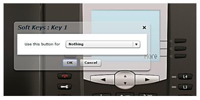
Use the drop-down list to select the operation that key should perform and configure. See the *Key Options* section 6.1.3 for a list of some of the available features.
