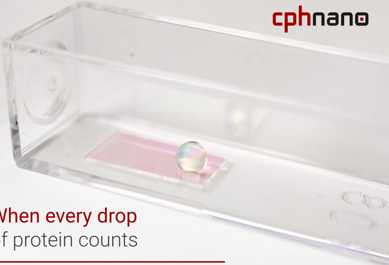
A clear, rectangular NanoCuvette One cuvette is shown at an angle. Inside, a small, flattened, iridescent droplet of liquid sits on a pink optical filter. The droplet shows rainbow-like colors due to light interference.
