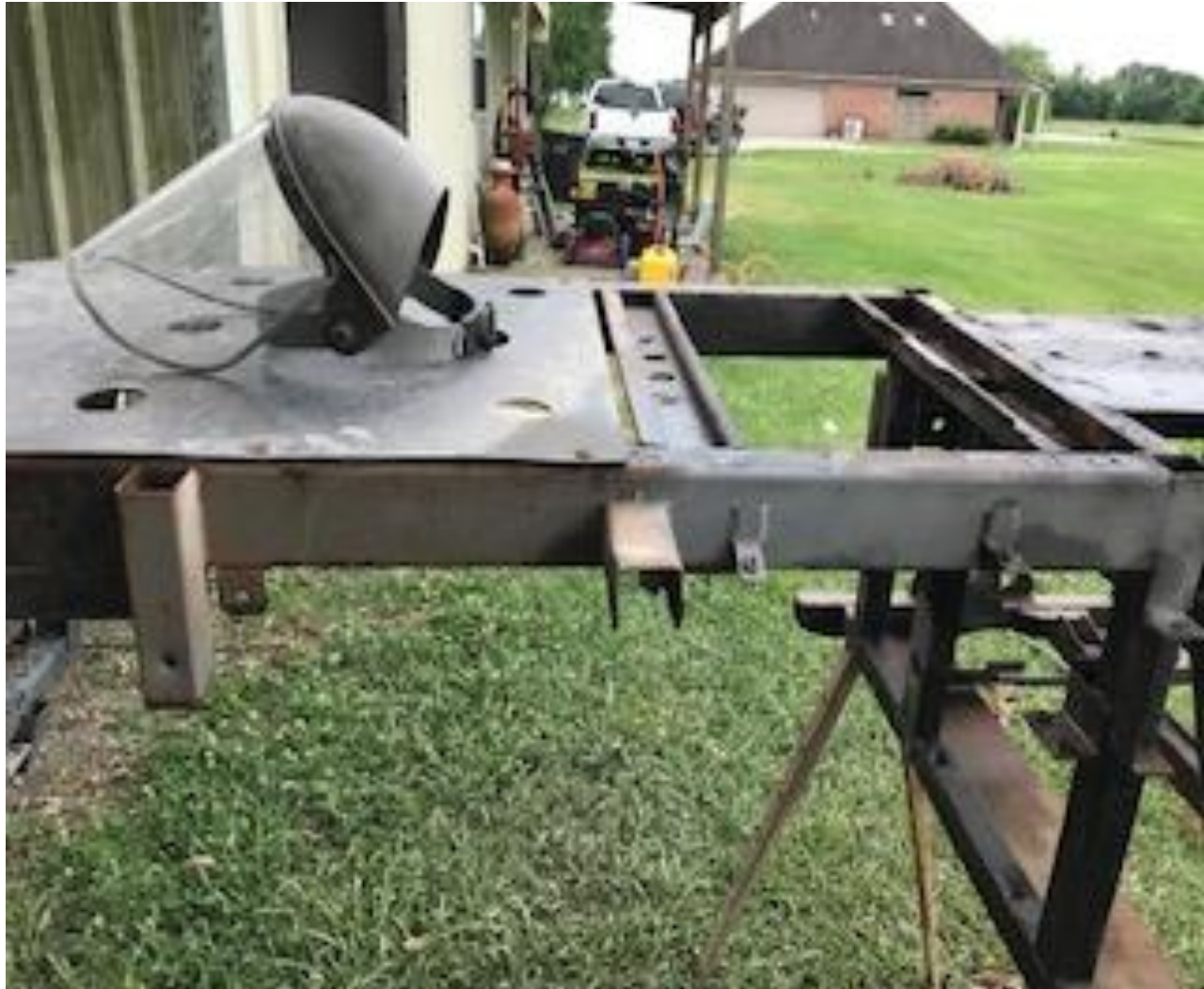
Corr-Ze 100™ rinse after Corr-Ze 200™ treatment
