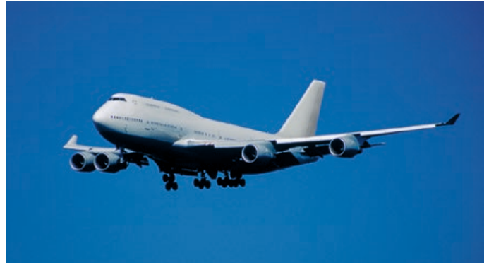
A modern passenger plane has a pressure complying with about 2500 m (or ca. 15.5% O 2 ).
