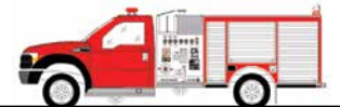
DARLEY VISION INITIAL ATTACK IA011 (CAFS Option Included) Pump (1000) 350 Gallon Tank Copolymer Attack Body
