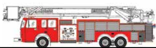
DARLEY VISION 104 AERIAL PLATFORM AR006 (CAFS Option Included) Pump (1000-1750) 300 Gallon Tank Copolymer Aerial Body
