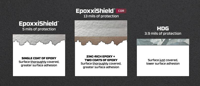
The high performance, fast-dry epoxy coatings range from a single layer of two-component polyamide epoxy in the EpoxxiShield<sup>™</sup> Standard package, to EpoxxiShield<sup>™</sup> COR Elite, which provides the ultimate protection in any environment.
