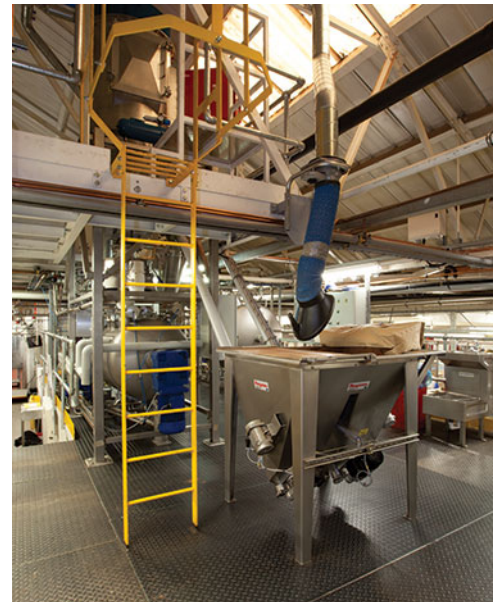
Two cocoa powders are transferred from the twin hopper through each flexible screw conveyor to the mixer, while sugar enters the mixer from pneumatic receiving hopper above. The entire batching/blending process is controlled by PLC.
