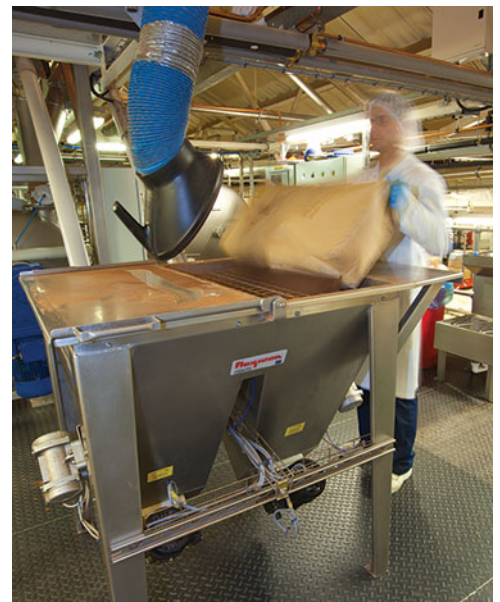
Two cocoa powders are transferred from the twin hopper through each flexible screw conveyor to the mixer, while sugar enters the mixer from pneumatic receiving hopper above. The entire batching/blending process is controlled by PLC.
