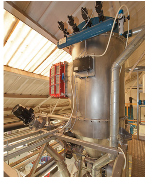
Sugar is fed into the mixer below from the 500 kg pneumatic receiving hopper. At left, cocoa powder enters the mixer through the discharge end of the flexible screw conveyor and downspout.
