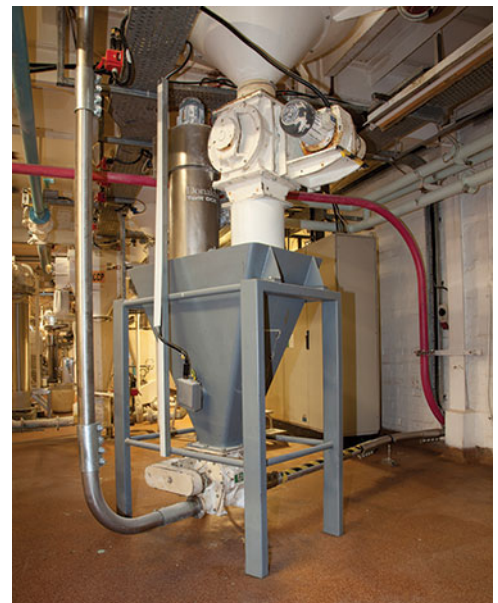
Two types of cocoa powder are emptied into the twin hopper while dust is removed by vacuum. The two flexible screw conveyors move each powder, alternately, to the mixer.
