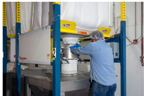
Two forklift-loaded bulk bag dischargers feed lentils to each floor hopper from which a flexible screw conveyor transports the lentils through the wall into the Packaging Room.
