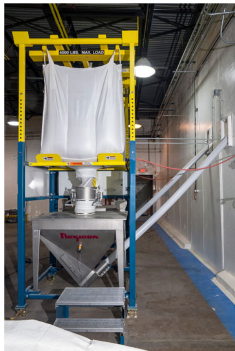
Two forklift-loaded bulk bag dischargers feed lentils to each floor hopper from which a flexible screw conveyor transports the lentils through the wall into the Packaging Room.
