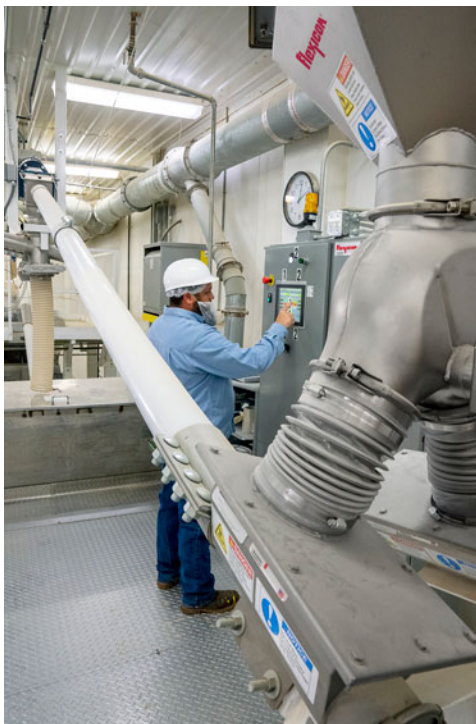
Interconnected flexible screw conveyors, under PLC control, deliver precise weights of lentils to four mixers.
