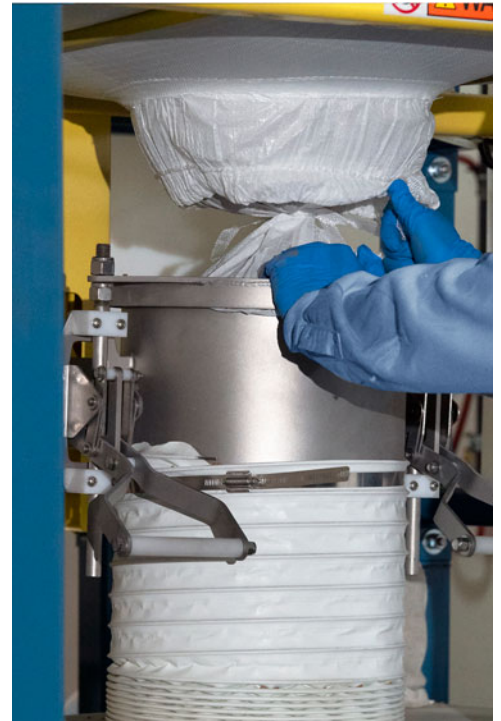
The SPOUT-LOCK® clamp ring positioned atop the TELE-TUBE® telescoping tube applies constant downward tension as the bag empties and elongates for full and dust-free evacuation.
