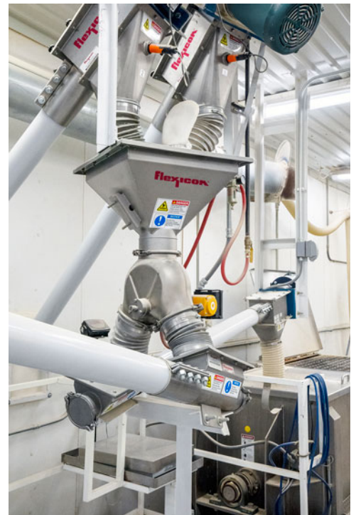
The SPOUT-LOCK® clamp ring positioned atop the TELE-TUBE® telescoping tube applies constant downward tension as the bag empties and elongates for full and dust-free evacuation.
