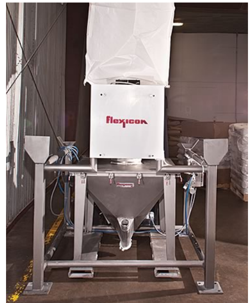
Limited headroom requires a forklift to suspend bulk bags above the lower half of this split-frame BULK-OUT® bulk bag discharger. Once the room is enlarged with a higher ceiling, bulk bags will be loaded at floor level into the top half of the split-frame, which will then be forklifted with bag intact, onto the lower half of the frame, within inches/centimeters of the ceiling.
