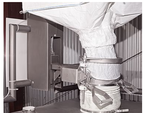
A SPOUT-LOCK® clamp ring secures the clean side of the bag spout to the clean side of a TELE-TUBE® telescoping tube, which maintains constant downward tension on the bag as it empties and elongates, promoting complete discharge.
