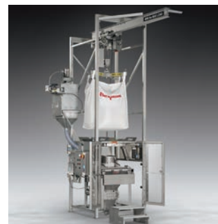
Sanitary BULK-OUT® Bulk Bag Dischargers create a dust-tight connection between the clean sides of the bag spout and the equipment, and collapse empty bags dust-free. Discharger frame, POWER-CINCHER® flow control valve, SPOUT-LOCK® clamp ring and TELE-TUBE® telescoping tube available USDA accepted.
