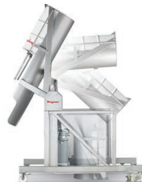
Open Chute Drum Dumper offers a low cost method of discharging free- and non-free-flowing bulk solids when dust generation is not a concern. Discharges directly into process equipment or optional hoppers equipped conveyor adapters or universal flanges.
