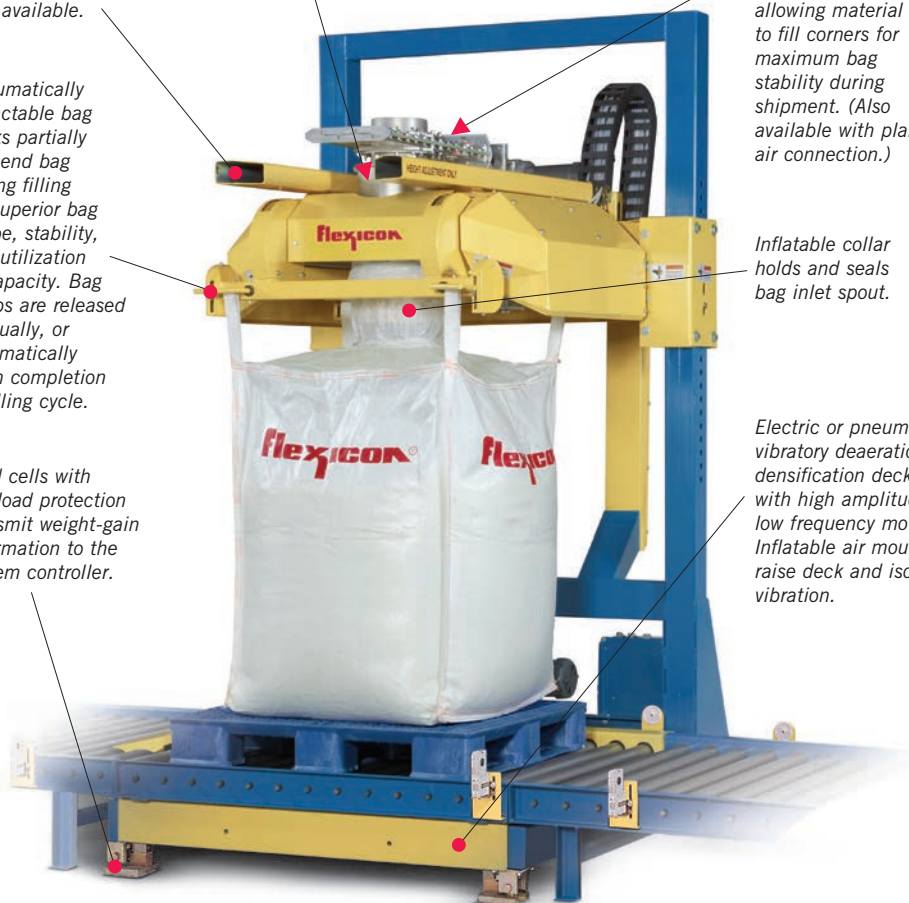
Flexicon's Low Profile Bulk Bag Filler allows removal of loaded bags using a pallet jack, eliminating the need for a forklift.
