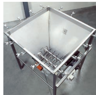
Flexicon offers a multitude of mechanical and pneumatic hopper accessories to promote the flow of poor-flowing or non-free-flowing materials. This hopper features dual agitators with interlocking paddles that de-agglomerate bulk material, promoting void-free charging of mechanical conveyor intake adapters.
