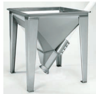
Divergent angles of Flexicon's high flow hopper design reduce the ability of non-free-flowing materials to establish a bridge between the hopper sidewalls, instead causing material to topple and flow toward and down the steep backwall, increasing the flow of bulk materials while decreasing residual material in the hopper.
