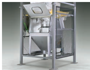
The Dust Containment Enclosure contains spillage and dust that can escape through seams in the bag and folds in the spout. The six-sided enclosure is equipped with an exhaust port for dust collection and a hinged door with inspection window.
