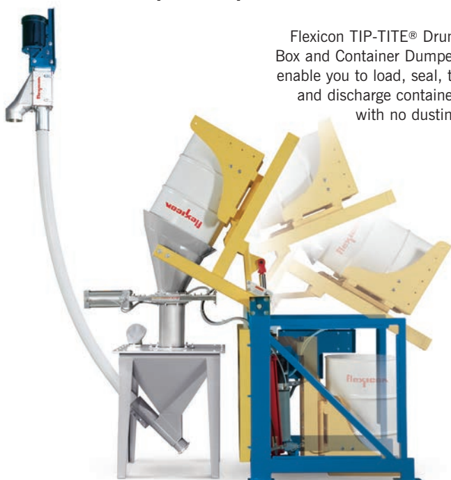
TIP-TITE® Universal Drum Dumper handles drums from 30 to 55 gal (114 to 208 liter). Shown with optional hopper configured with Flexicon flexible screw conveyor. Also available with hopper configured with Flexicon pneumatic pick-up adapter, or universal flanged outlet.
