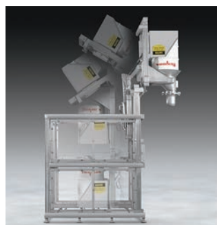
Sanitary TIP-TITE® Drum Dumpers allow loading, sealing, tipping and discharging of drums with no dusting by forming a dust-tight seal between a drum discharge cone and a gasketed receiving ring fitted to existing process equipment or the lid of a hopper.
