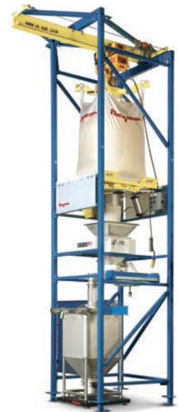
Flexicon's Bulk-Bag-to-Rigid-Bin Weigh Batching System seals against the clean side of the bag spout, elongates the bag for total evacuation, and allows dust-free retying of partially empty bags. A low-profile de-lumping device breaks up agglomerates as a gravimetric feeder loads accurately weighed batches into rigid bins.
