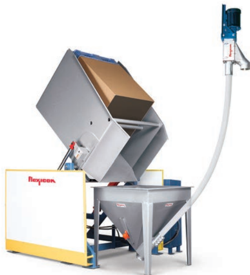
Flexicon Open Chute Box/Container Dumper handles containers up to 48 in. W x 48 in. D x 44 in. H (1220 mm W x 1220 mm D x 1120 mm H). Shown with optional hopper configured with Flexicon flexible screw conveyor. Also available with hopper configured with pneumatic pick-up adapter, or universal flanged outlet.
