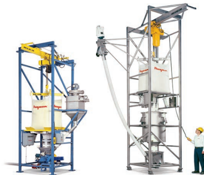
Flexicon Bulk Bag Continuous Loss-of-Weight Dischargers feature an activated surge bin and flexible screw conveyor, allowing continuous loss-of-weight (gravimetric) feeding directly from bulk bags. System software switches to volumetric mode during bag changes.
