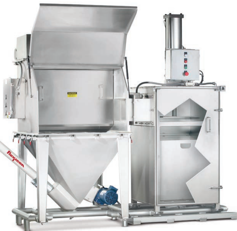
Self-contained Bag Dump System integrates a dust collector, flexible screw conveyor and bag compactor on a skid, streamlining installation and allowing easy relocation. The entire airtight system is under negative pressure, containing dust when bags are dumped, as well as when empty bags are pushed through the chute and compacted.
