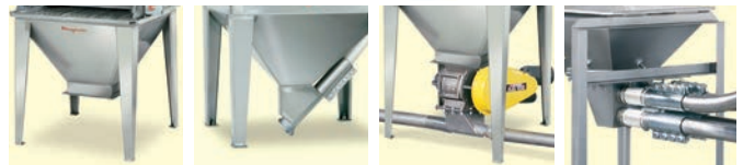
The hoppers of Flexicon Bag Dumping Stations are offered with outlets configured for: (left to right) direct connection to process equipment, flexible screw conveyor charging adapters, rotary airlock valves with flow-through adapters, and non-flow-through pick-up adapters for multiple conveying lines.
