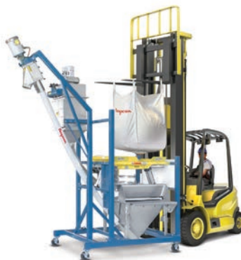
This Mobile Half-Frame Bulk Bag Unloader with multi-purpose hopper allows material to be discharged from bulk bags suspended from forklifts or hoists, manually dumped from sacks, and conveyed to equipment and storage vessels—dust free.
