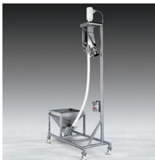
Sanitary Flexible Screw Conveyors are totally enclosed, preventing plant and product contamination. The inner screw connects to the motor drive beyond the material outlet, eliminating material contact with bearings. Tool-free disassembly. USDA accepted and 3-A certified.
