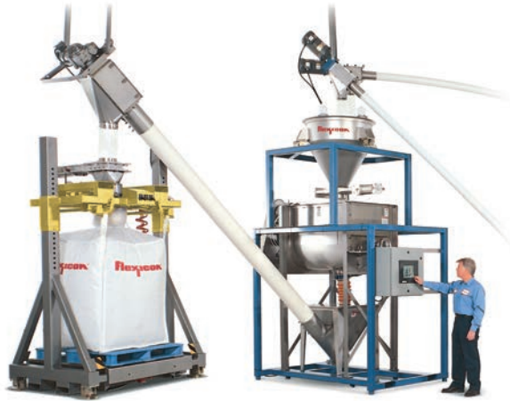
Flexicon's Self-Contained, Gain-in-Weight Batching and Blending System conveys bulk ingredients from multiple upstream sources, weigh-batches, blends and discharges the material into a surge hopper, and transports it to a TWIN-CENTERPOST™ Bulk Bag Filler. The system is offered with Flexicon Flexible Screw Conveyors (shown) or PNEUMATI-CON® Pneumatic Conveying Systems.
