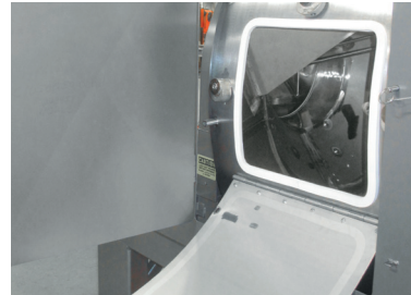
Large doors provide unrestricted access to the wide-open vessel interior for cleaning and inspection.
