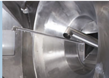
Large doors provide unrestricted access to the wide-open vessel interior for cleaning and inspection.
