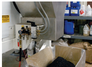
Rotary Batch Mixer shown discharging one of 200 blends of tea with no cross contamination.
