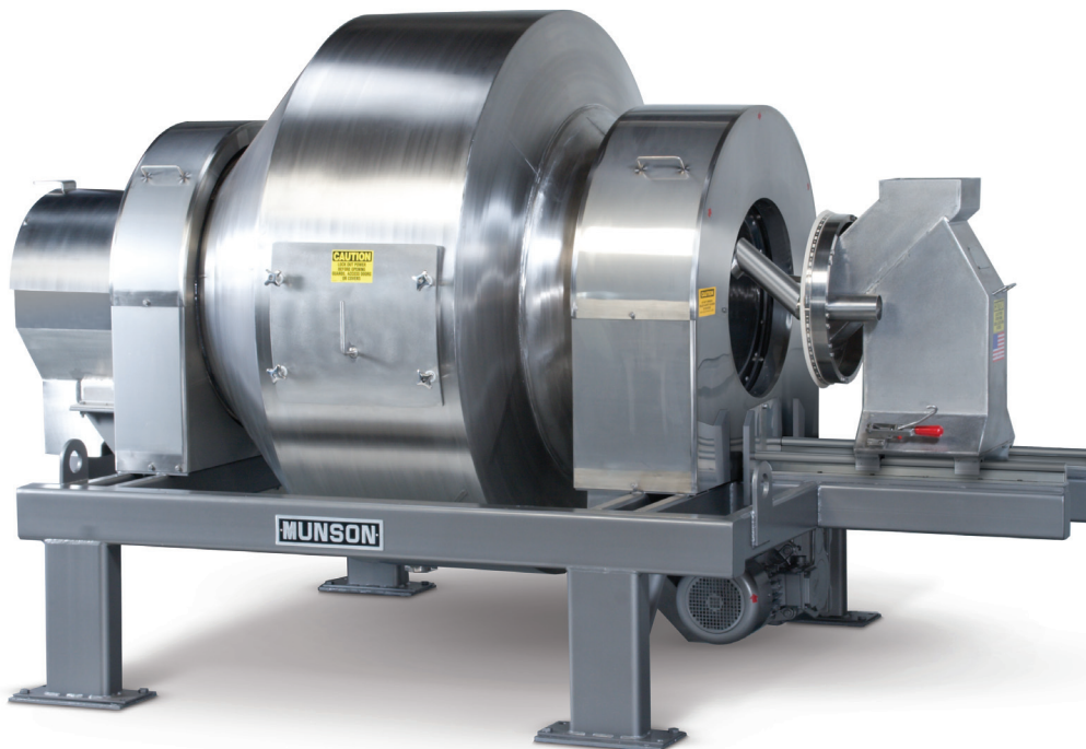
Rotary Batch Mixers are available in useable capacities to 600 cu ft (17 cu m). Shown is a 40 cu ft (1.13 cu m) sanitary stainless steel model with retractable inlet, for blending of spices.
