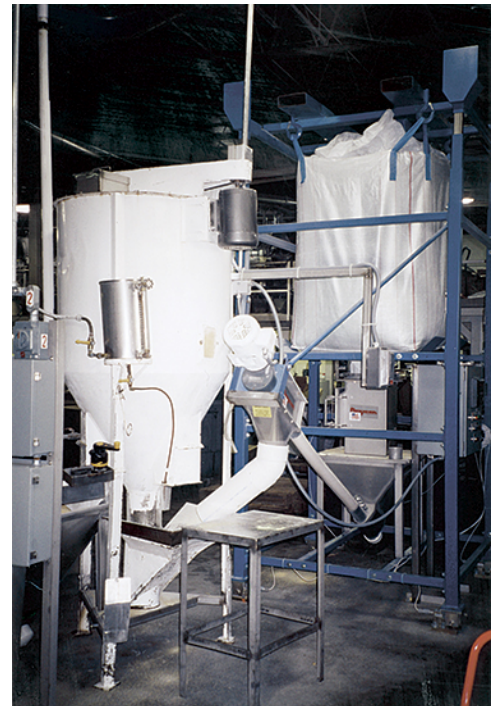
Bulk bag unloader with 2000 lb bag of cornmeal discharges into hopper equipped with flexible screw conveyor which transports the material to a vertical blender where it is moisturized.
