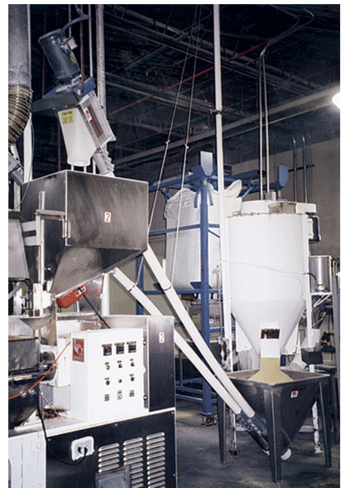
Bulk bag discharger with flexible screw conveyor is mounted on load cells that transmit loss-of-weight information to a controller which stops the conveyor once the target batch weight is discharged.
