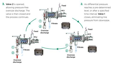
**Reduce time and labor** – No need to monitor filter and open oversize discharge valve.
