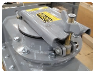
Cleanout ports to inspect for product in the lower air chamber and maintain, if necessary. Each section of the conveyor has a cleanout port, located along the bottom of the lower air chamber.
