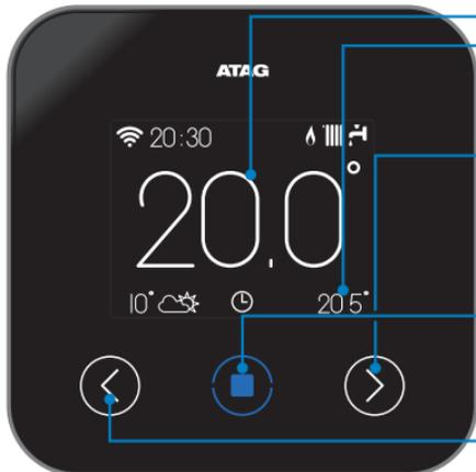
The diagram shows a black ATAG ONE<sup>Zone</sup> thermostat with a color display. The display shows the time 20:30, a Wi-Fi signal, a flame icon, a battery level icon, a large temperature of 20.0, a weather icon, a clock icon, and a setpoint of 20.5. Below the display are three touch-sensitive buttons: a left arrow, a central blue square, and a right arrow. Blue lines connect these elements to callout boxes on the right.
