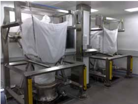
BBDL's low clearance is ideal for cleanrooms with HVAC systems in the ceiling.
