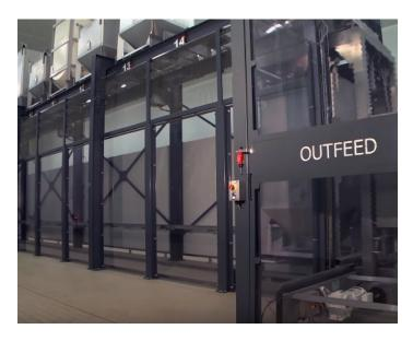
'Ingredient' containers are located on the framework, with 'batch' containers travelling below collecting ingredients according to the batch recipe
