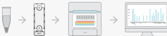
Figure 3 | The IsoLight automated benchtop system requires only five minutes of hands-on time, compared to conventional multiplexed bulk cytokine ELISA platforms which require six to ten hours of hands on time for the user. All ELISA procedures are automated on the IsoLight, and data is fully analyzed via IsoSpeak software.
