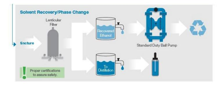
The final distillation removes any remaining unwanted materials, such as lipids, waxes, cannabinoids, chlorophyll, terpenes and other impurities. The final distillation phase creates the golden final product that is clear, bright and enjoyable.
