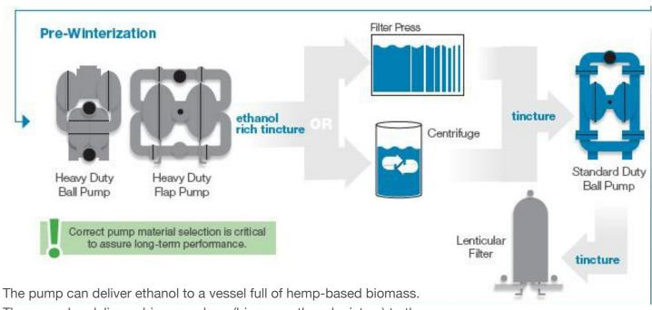
They can also deliver a biomass slurry (biomass ethanol mixture) to the vessel using the AODD pump for winterization and extraction.
