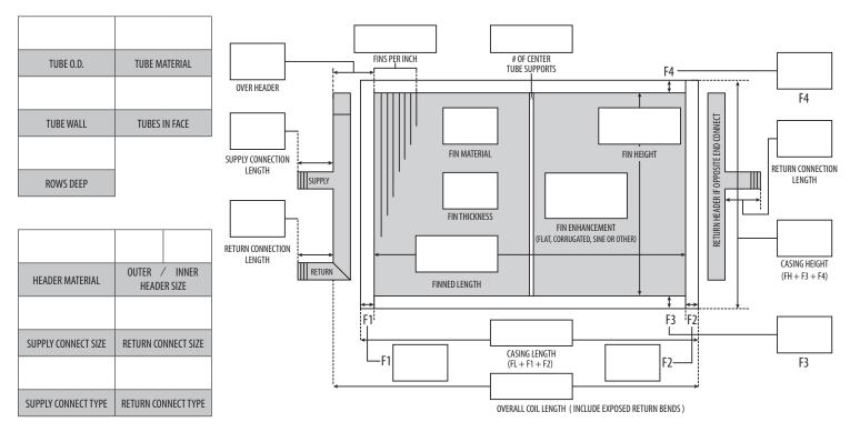
NOTE: INNER HEADERS MUST BE GREATER THAN SUPPLY CONNECTION SIZE. OUTER/RETURN HEADER MUST BE GREATER THAN INNER HEADER
