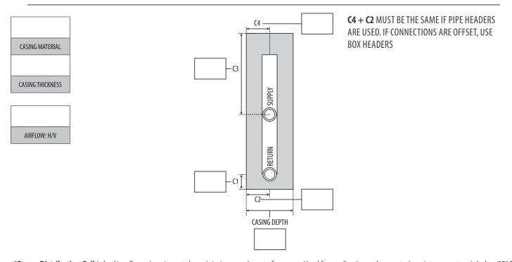
\*Steam Distributing Coil (a.k.a Non-Freeze), an inner tube; minimizes condensate freeze up. Used for applications where entering air temperature is below 32° F. Provides even air temperature on long coil lengths when steam is modulated, and /or supply and return connections must be on the same end of coil.
