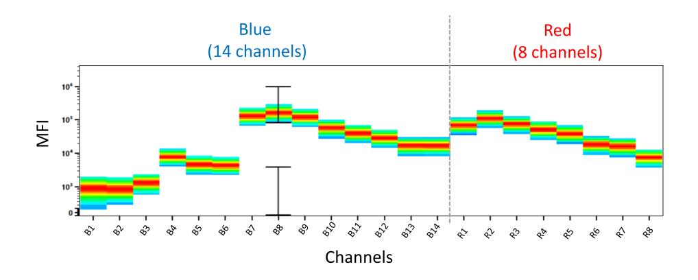
This dye is excited by both lasers. The peak channel (indicated by the black bar) is in channel B8, and it has secondary emission in channel R2. Based on this information, expect this dye to introduce spread into dyes emitting at similar wavelengths.
