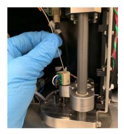
Slide the beige nut down into the hole and turn the nut to secure, but do not tighten.
