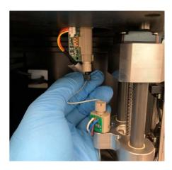
Follow the tubing from the black nut down to the beige plastic nut. Twist off the beige nut and gently pull it and tubing out from the SIP.
