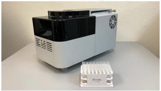
The ASL resuspends samples using an orbital shaker. In addition to supporting a variety of 96-well plates, including deep-well plates, it supports a 40-tube rack. Loader settings are user-adjustable, including mixing speed, mixing duration, the number of SIT flushes between samples, and data record delay time. Loader settings are Default (standard), High throughput, and Low carryover.
