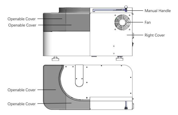
The Manual Handle is located on the right side of the Loader. The handle is a mechanical lever used to make the instrument work in Plate Mode, Tube Mode, or Tube Rack Mode. The handle can be moved with either power on or power off.
