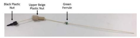
Open the SIT door. Identify the three components shown in the following figure.
