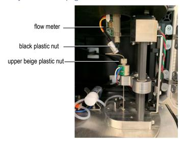
Twist off and carefully remove the black plastic nut from the bottom of the flow meter.
