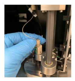
Mark the fully screwed in position at the base and on the nut, as shown. Then unscrew the nut 1½ revolutions from the marked position.
