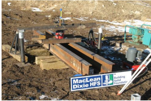
Full scale field testing-compression/tension/lateral
