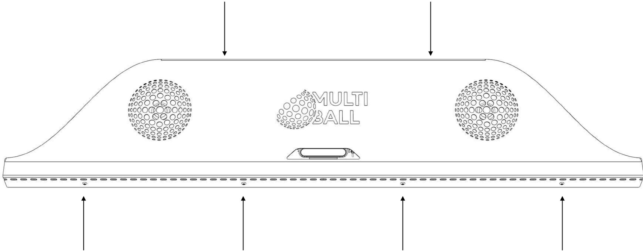
**i** Remove the 6 screws and lift up the cover.
