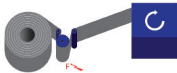
Version 211: Electromagnetic friction adjustable from control panel.
